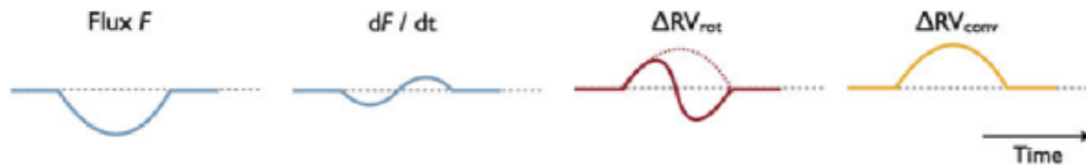
Fig. 2.10 The FF' method for a spot crossing the stellar disc. The RV variations induced by flux blocking ( \Delta RV_{\text{rot}} ) and suppression of the convective blueshift ( \Delta RV_{\text{conv}} ) are proportional to F dF/dt and F^2 , respectively. Fig. By Haywood
